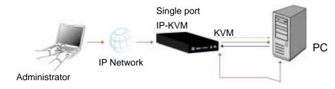
Figure 3-1.a: IP-KVM switch usage scenario
